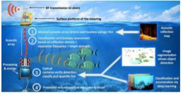
Image source: Principle of operation of the SYMBIOSIS autonomous opto-acoustic system, <u>http://symbiosis.networks.imdea.org</u>
